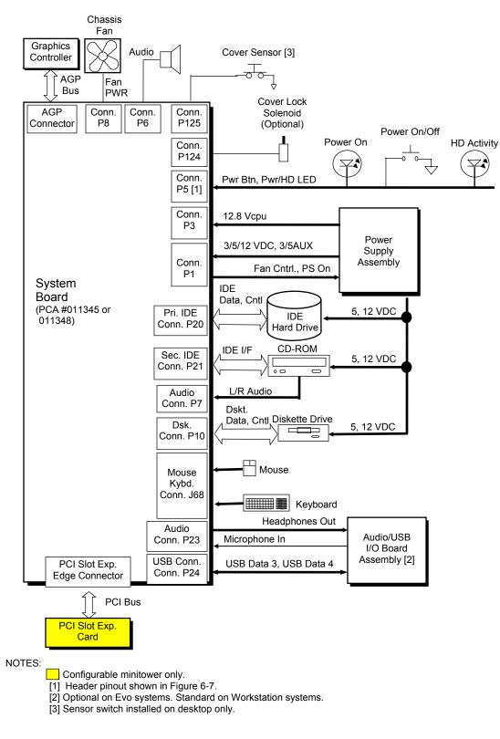
Figure 6–6. Desktop/Minitower Signal Distribution Diagram
